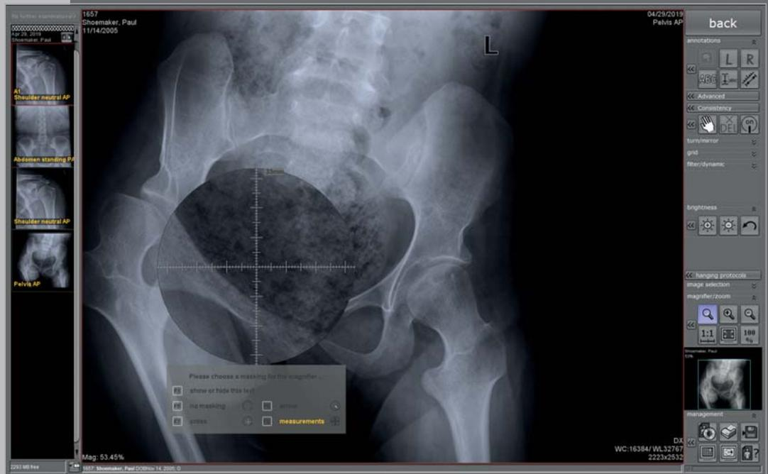
The stitching module creates a single image from separate digital X-ray images (optional)
