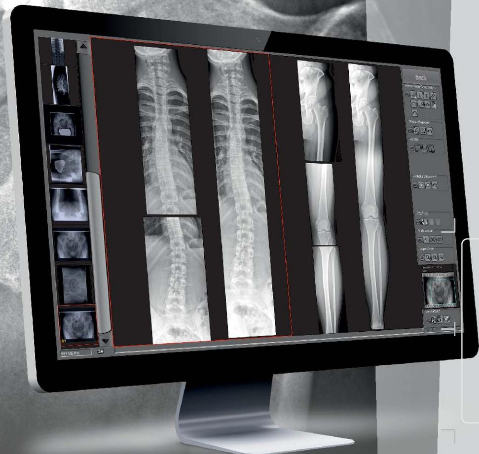
The **stitching module** creates a single image from separate digital X-ray images. The images are loaded, correctly aligned and merged to one image.
